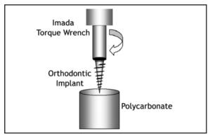
Fig. 2 Miniscrew driven into polycarbonate rod with torque wrench.
